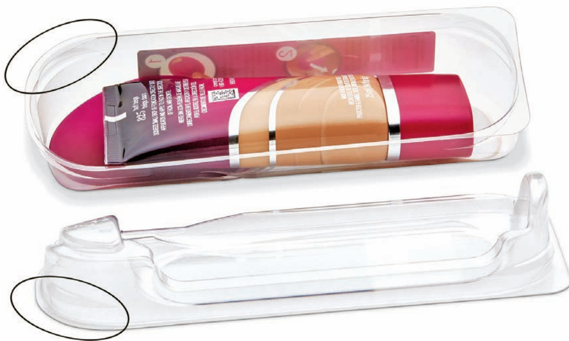
The undercut design (circled) allows the blister lid to snap into the base to secure the package without heat sealing or RF welding. The same undercut allows the bases, and the lids, to stack rather than nest for easy denesting on the packaging line.
