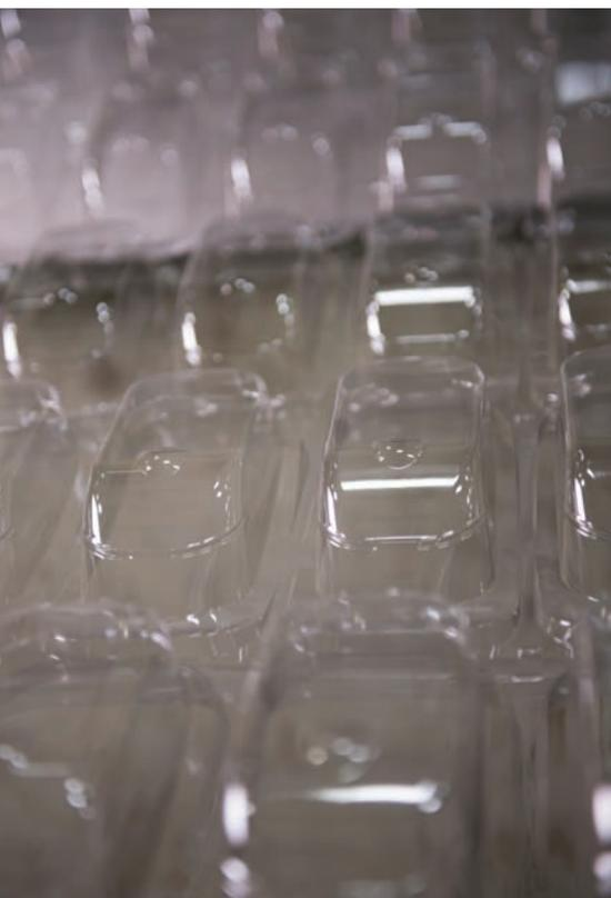
The blister's easy-open design includes a fingertip-shaped opening flanked by perforations. Placon thermoforms the blister from PETG.
